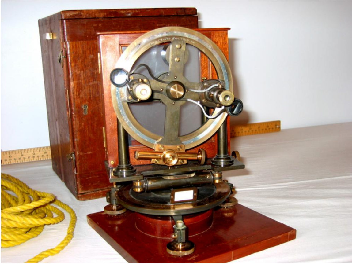
Figure 2: Dover Dip Circle, an instrument for measuring the inclination during early 20 th century magnetic surveys. While innovative for its era, instruments like this required a high level of skill and patience from its users. The lack of modern materials and techniques meant even the smallest of errors could creep into the measurements.
